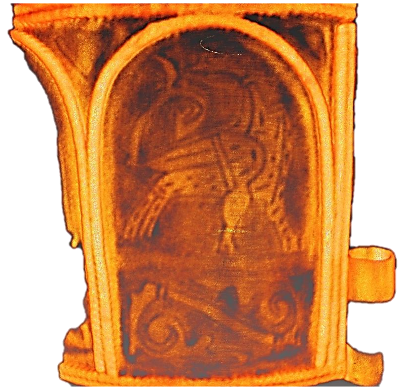
Neutron tomography reconstructed model with “hidden” gilding pattern of old-russian ancient bracelet dated to XIV century
