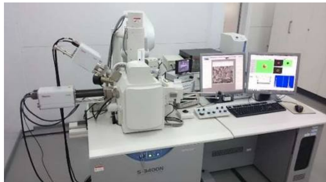
SEM Hitachi S3400N Resolution of 1 nm at 15 kV EDS, WDS Electron backscattering diffraction
