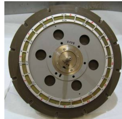
^{242}\text{Pu} 24-cm target wheel 12 sectors
