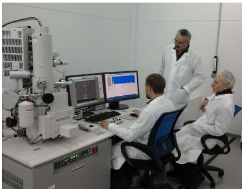
FESEM Hitachi SU8020 Resolution of 1 nm at 15 kV X-ray element microanalysis (EDS) Deceleration mode (500 eV)
