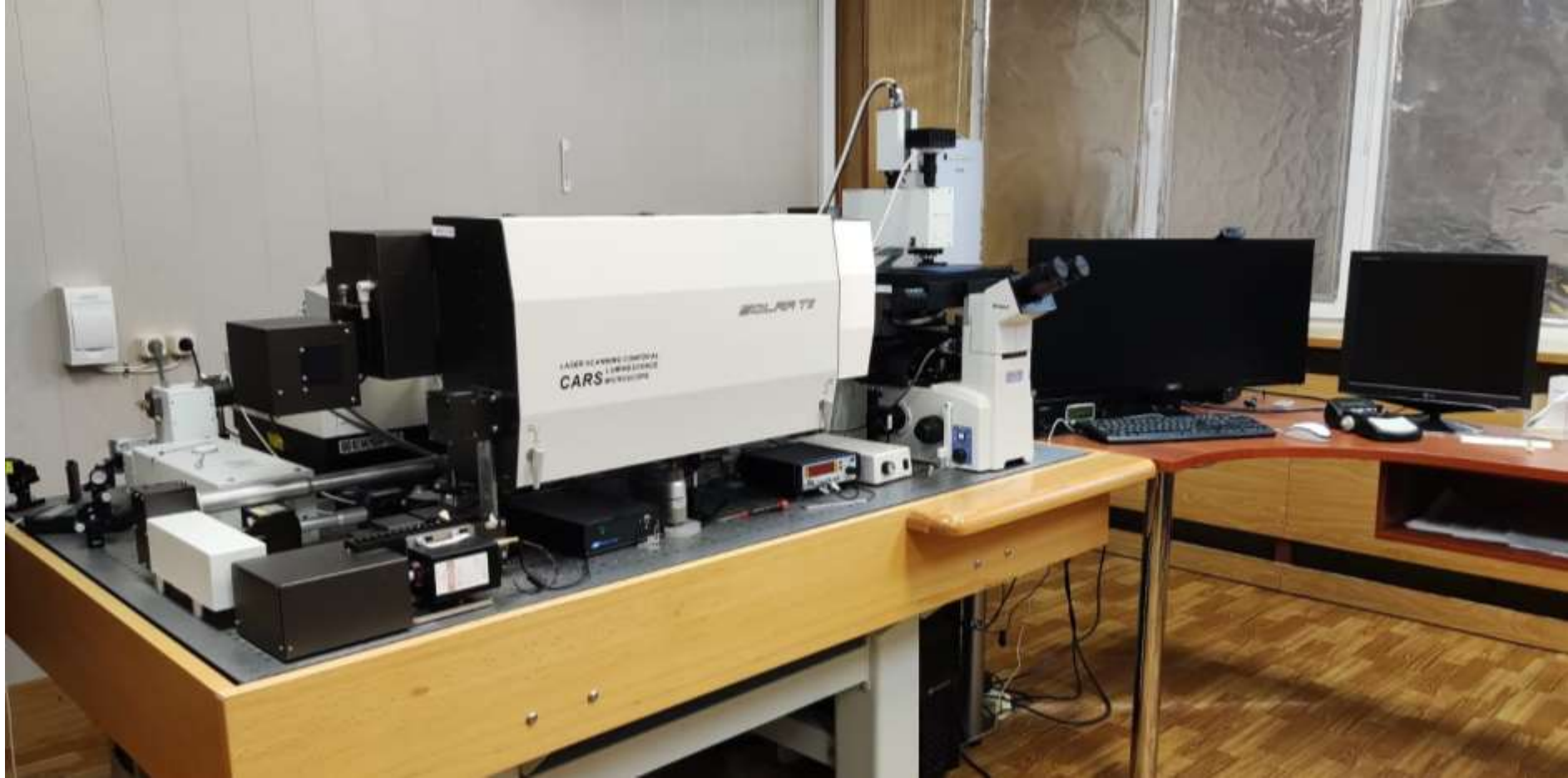
Fig.6. Laser scanning confocal luminescence microscope (with CARS) at the Department of Raman Spectroscopy, Frank Laboratory of Neutron Physics.
