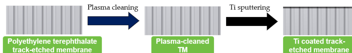
Fig.1. Production of hybrid/multifunctional membranes using 1 sputter target
