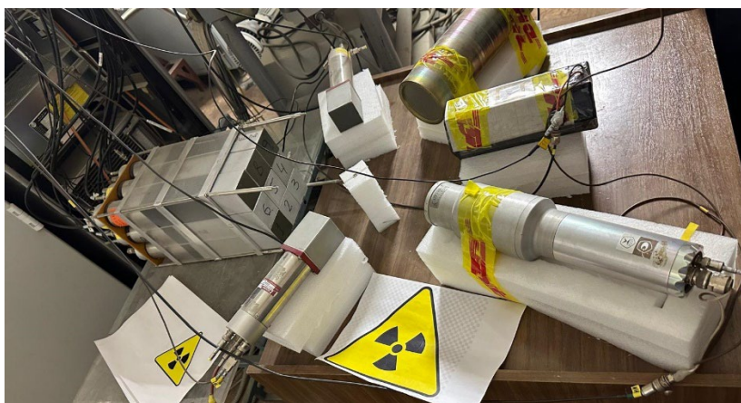
Fig. 4. The experimental setup for measuring the response function to neutrons and \gamma -quanta.
