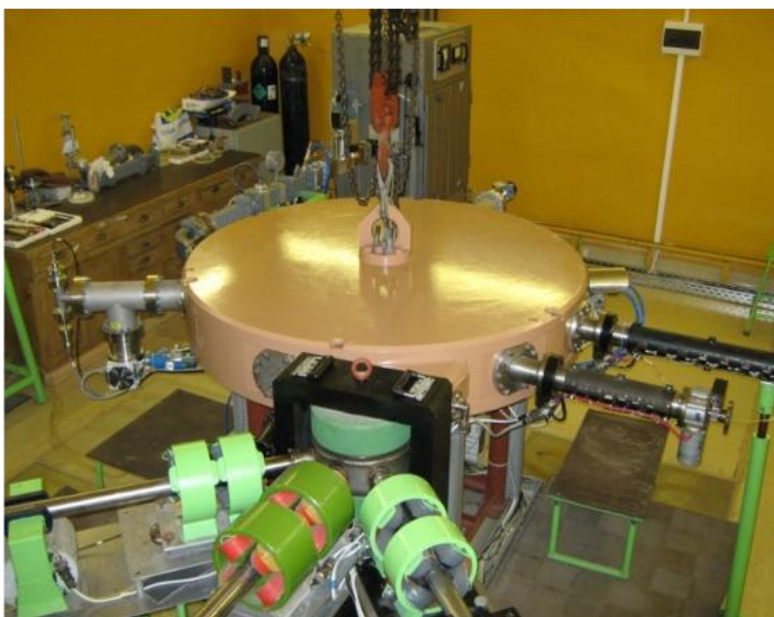
Figure 1. Microtron MT-25 (a) and HPGe spectrometer CANBERRA GC3018
