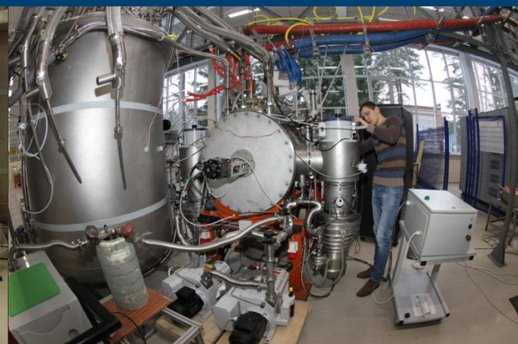
Tests of the pre-serial dipole magnet: magnetic field measurements
