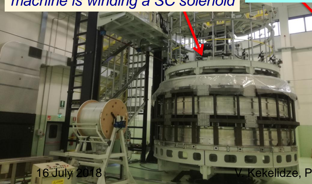
machine is winding a SC solenoid
