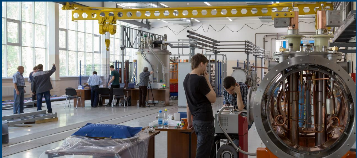
The technological line for SC magnet assembly and tests
