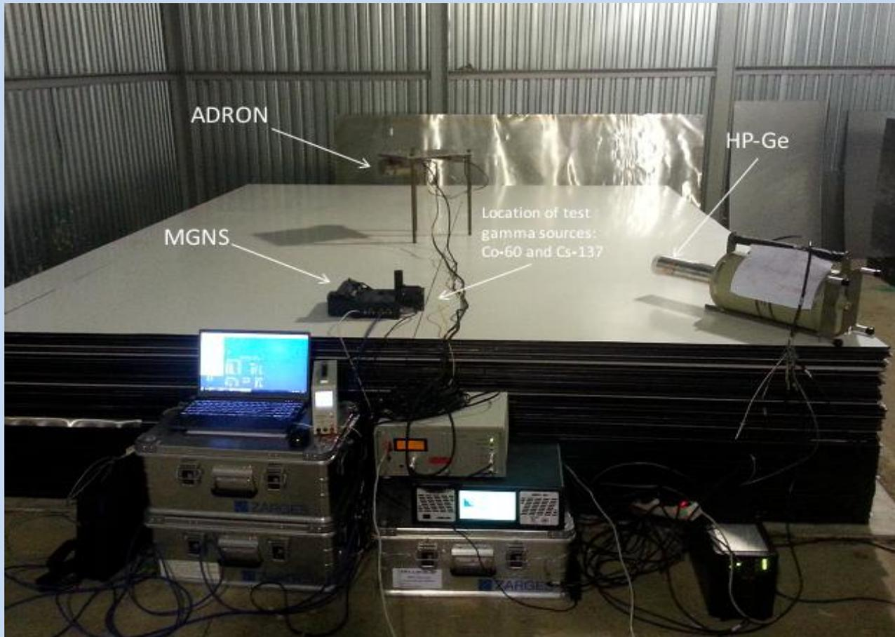
In collaboration between the Space Research Institute (RAS) and FLNP (JINR), a *special facility has been constructed* at the LRB that can *model planetary soil* and allows testing prototypes of active neutron and gamma spectrometers.
