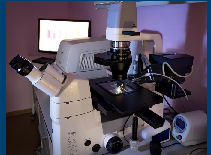
Zeiss AxioVert microscope with microinjection/micromanipulation system
