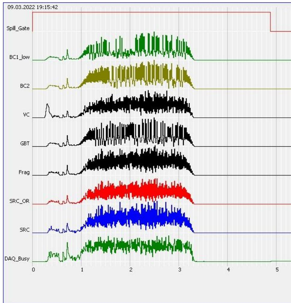
Intensities of the 3 GeV/u carbon beam as a function of time measured at the BM@N setup (SRC experiment) for one spill. X axis shows time in seconds.
