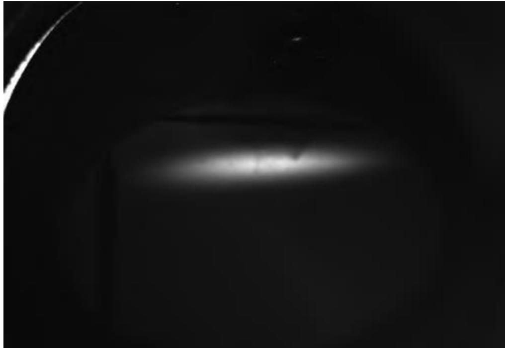
Beam of Fe ions on the phosphor screen
