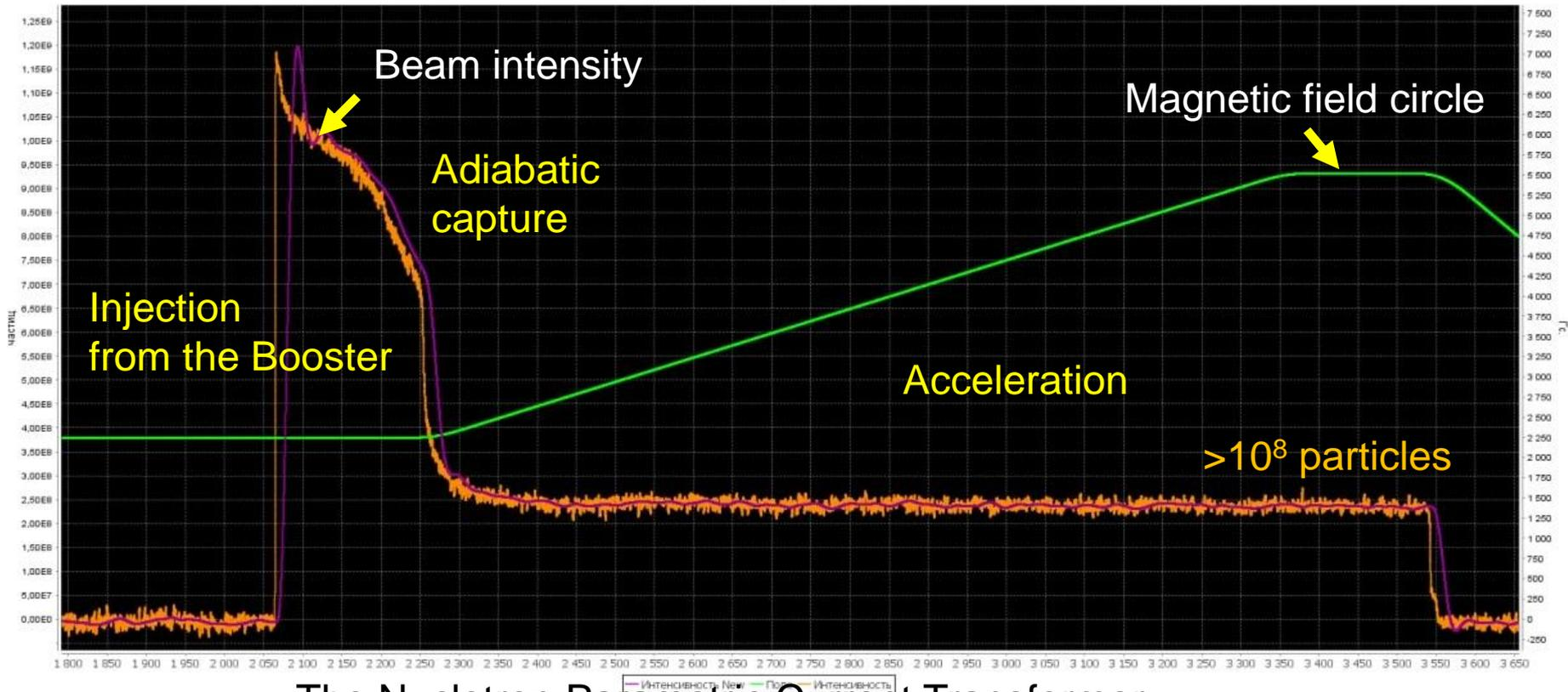
The Nuclotron Parametric Current Transformer
