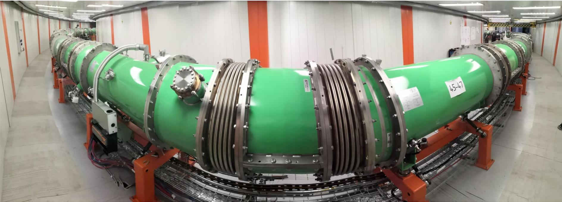
Cryo-magnetic system in assembly
