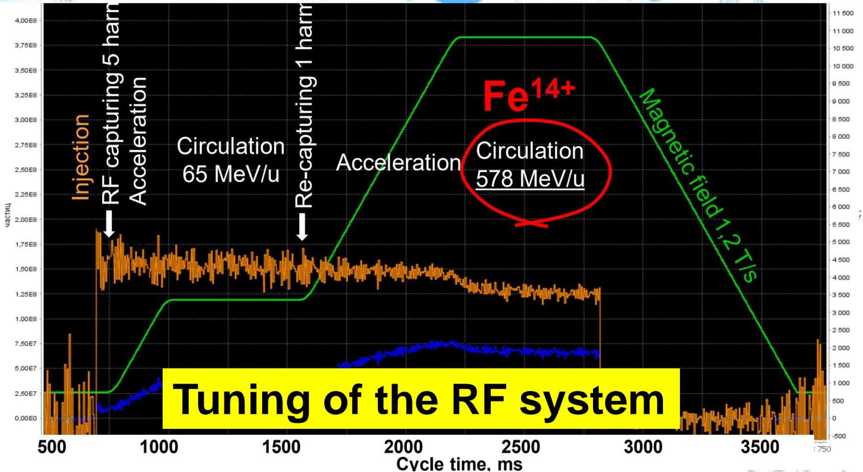
Adiabatic capture of the beam into acceleration was fulfilled at 5-th harmonics of the acceleration field,
