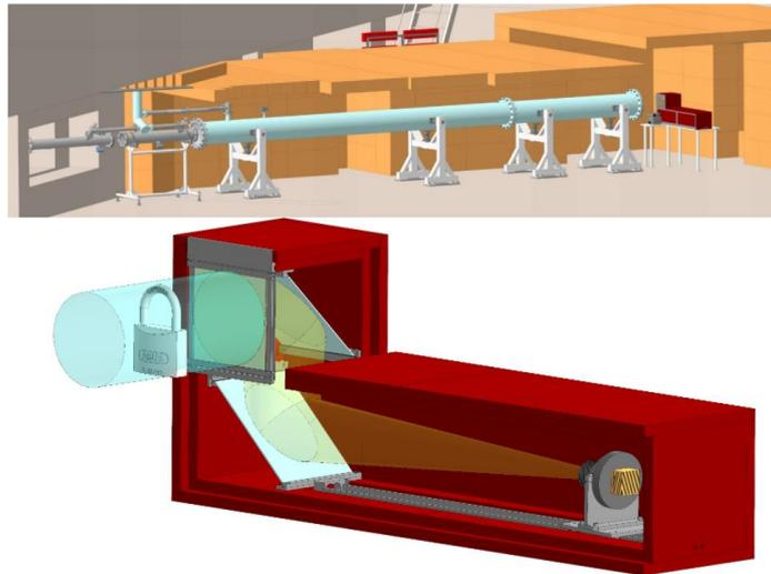
**Fig2.2.1** At the top: The layout of the neutron radiography and tomography facility on the 14th beamline of the IBR-2 high-flux pulsed reactor.
