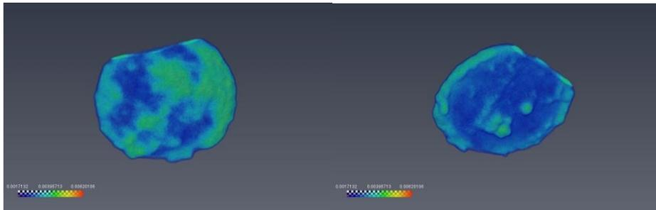
**Fig3.3:** The coin 467 visulaized in 3D in Avizo 8.1 after tomographic reconstruction.
