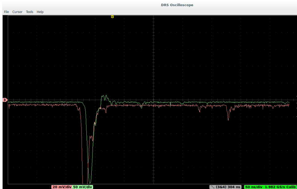
Figure 16: Coincidence counting from two plastic detectors
