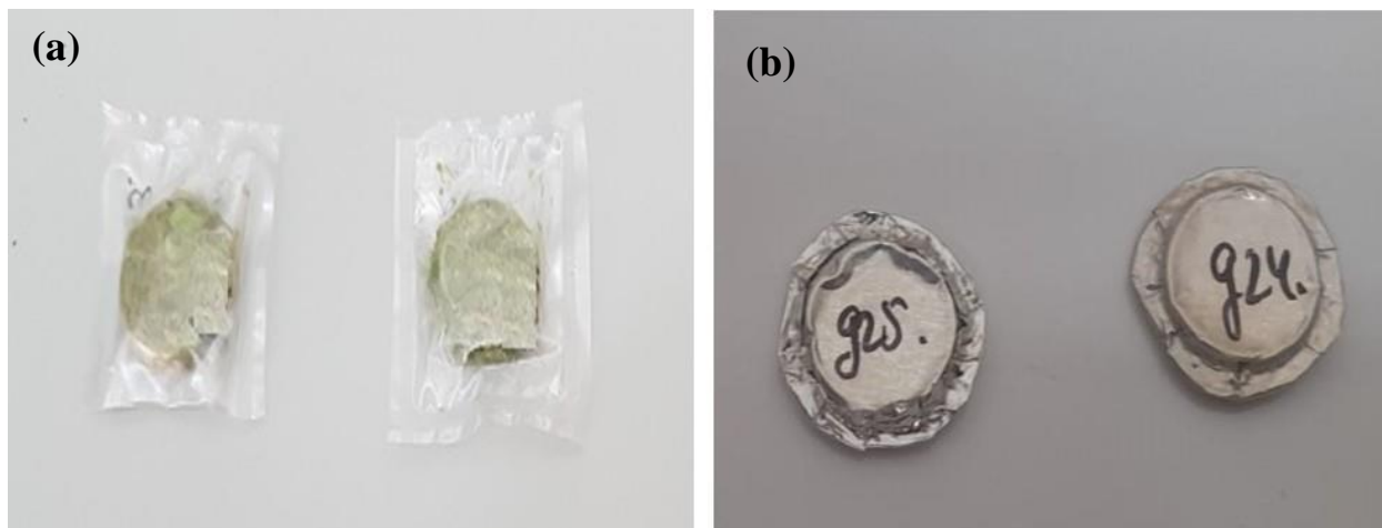
Figure 3 shows the third step in the sample preparation process: Moss samples were wrapped in (a) polyethylene bags and (b) aluminum cubs for short- and long-lived irradiations respectively.
