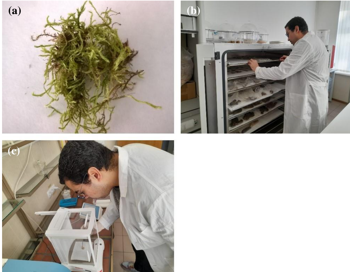
Figure 1 shows the first step in sample preparation process (a) collected moss sample, (b) drying samples in a drying oven, and (c) weighing samples to a constant weight.
