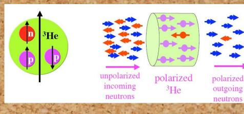
Polarized neutrons are a collection of neutrons whose spins have a preferential orientation with respect to a particular direction in space (usually the direction of a magnetic field), rather than being at random.
