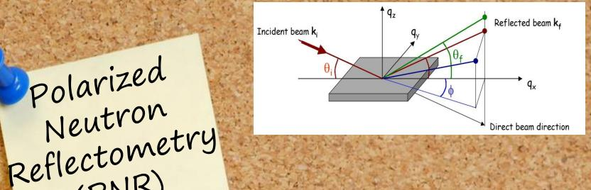
A method used to determine the structure of materials by directing a beam of polarized neutrons onto an extremely flat surface.
