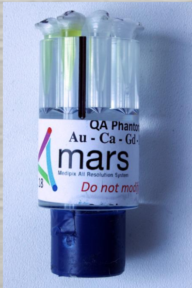
Phantom with 9 falcon tubes containing different materials
