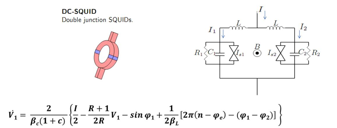
$$\dot{V}_{2} = \frac{2}{\beta_{c}(1+c)} \left\{ \frac{I}{2} - \frac{R+1}{2R} V_{2} - Ic \sin \varphi_{2} + \frac{1}{2\beta_{L}} [2\pi(n-\varphi_{e}) - (\varphi_{1}-\varphi_{2})] \right\}$$
