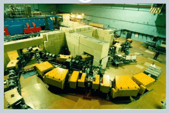
designed for separating and forming beams of unstable nuclei obtained in reactions with low- and intermediate energy (~40 MeV/u) heavy ions.
