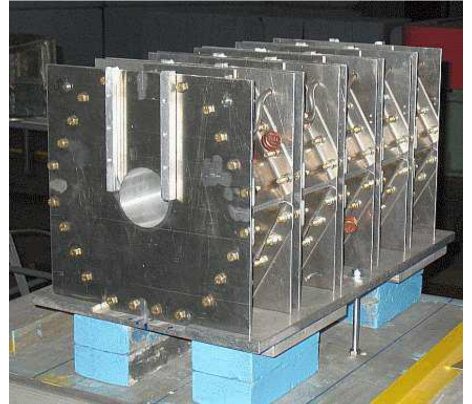
'Quinta' experimental set with lead shielding and the 'Quinta' assembly, with visible separated sections.
