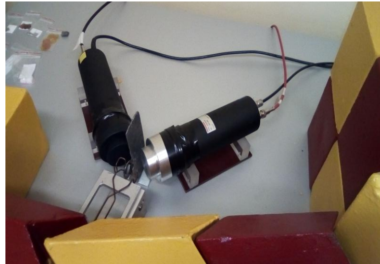
Titanium samples attached to two photomultipliers.
