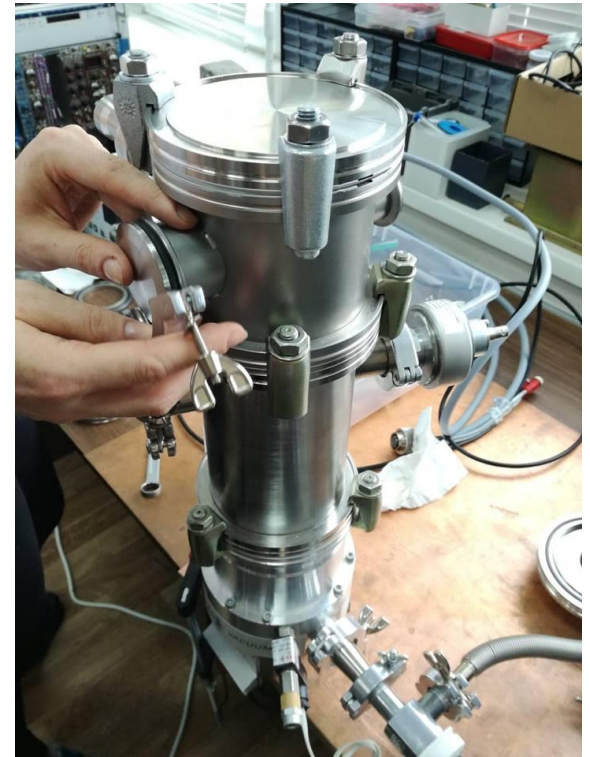
Assembling a vacuum chamber
