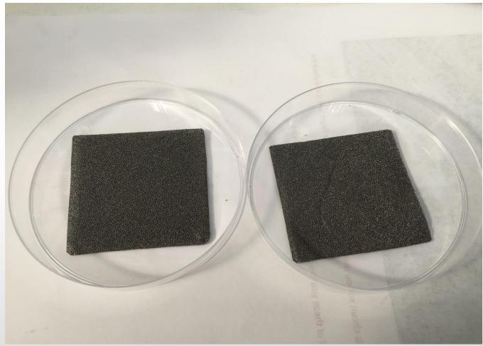
3D graphene (pure and with Ni foam as a template) and 3D graphene/ZnO composite networks were prepared by **chemical vapour deposition (CVD)** process with methane as the carbon source.
