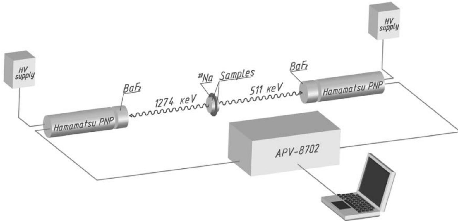
Positron lifetime spectroscopy apparatus
