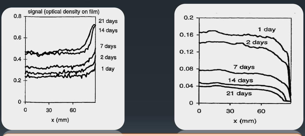
Distribution of moisture construction Obtained by signal transformation analysis
