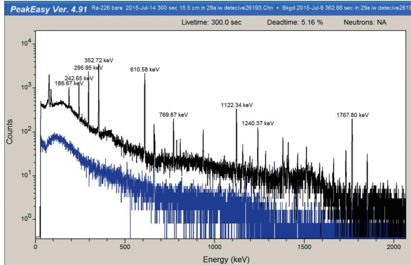
**Figure 7:** Spectrum of an unknown isotope and  $\gamma$ -ray radiation source.
