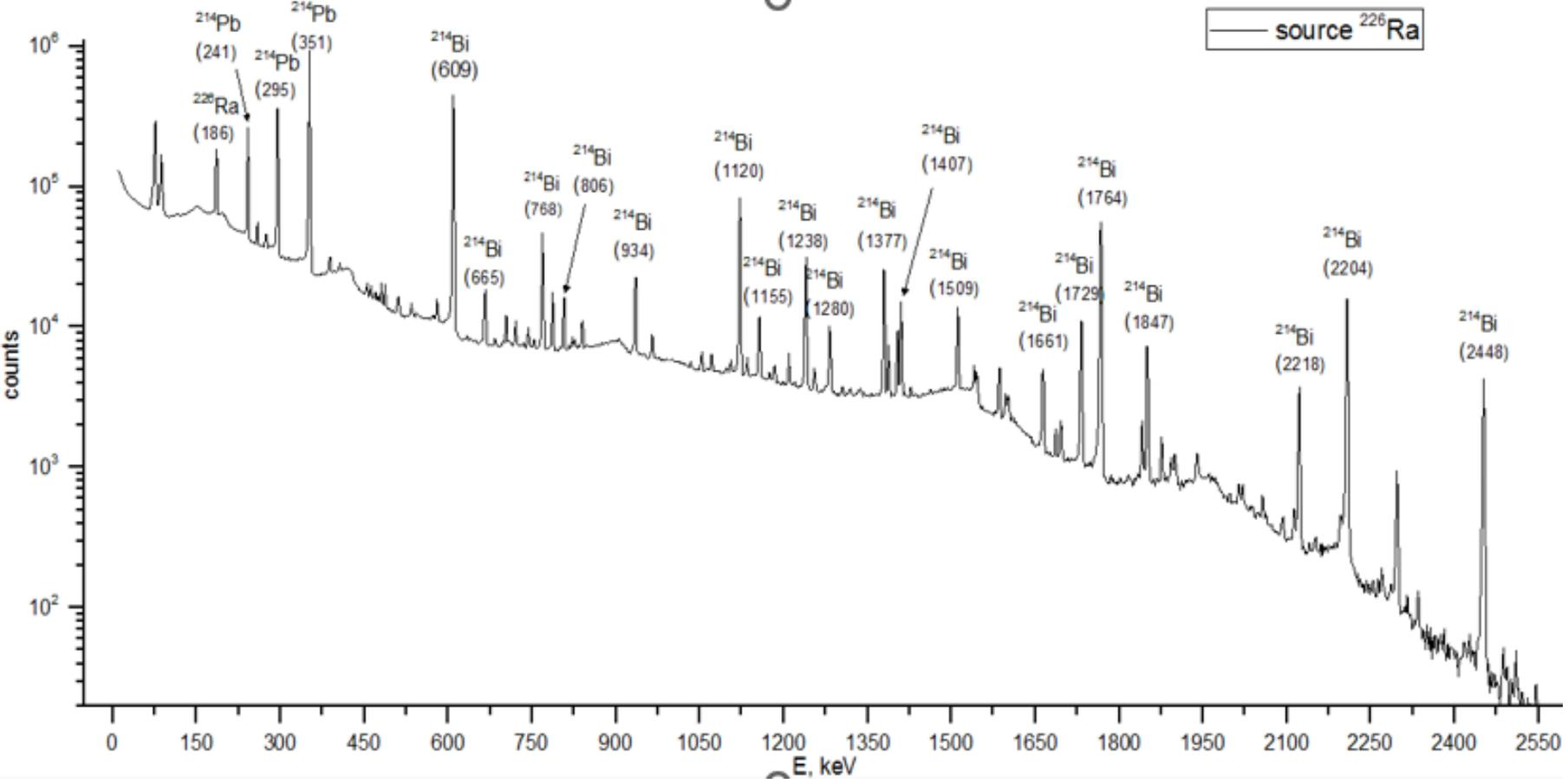
Figure 9: Identity and energy spectrum of the unknown isotope and radiation source
