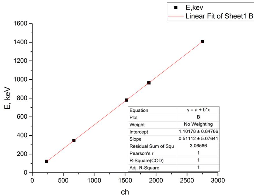
**Figure 3:** (a)GammaMCA program and (b)calibration line in Origin, where E is energy (keV), D is channels.
