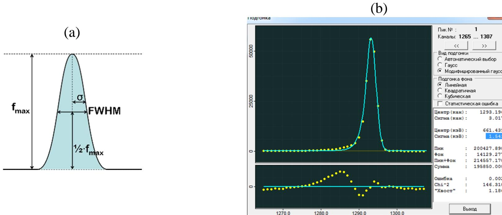
**Figure 4:** Energy resolution determination ((a), (b) graphical and analytical methods)
