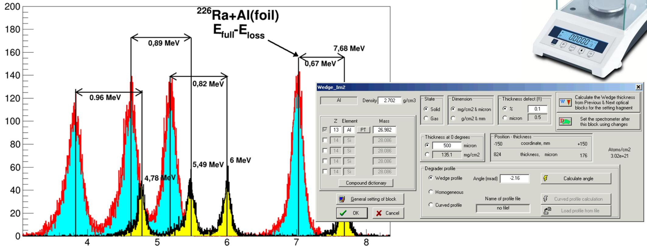
Figure 10: Energy loss calculation/foil thickness using Lise++ software
