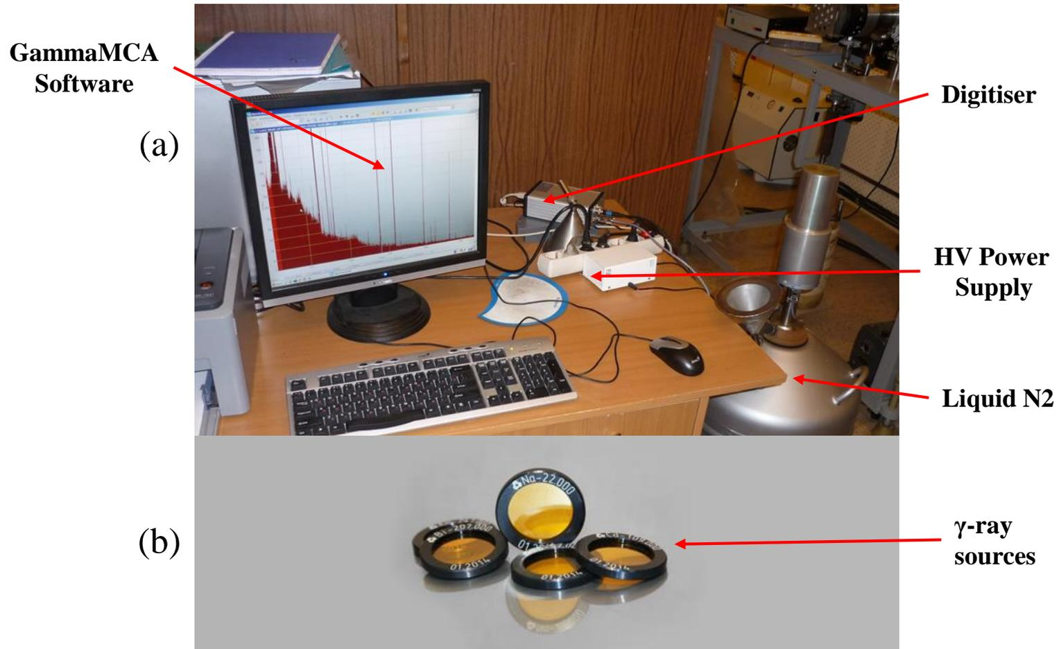
**Figure 1:** (a) Ge(Li) detector (a)workstation utilising GammaMCA software for real-time and offline viewing of  $\gamma$ -ray energy spectra and (b)  $\gamma$  radiation calibration sources
