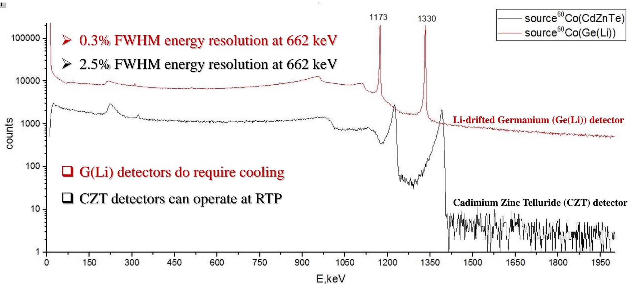
**Figure 6:** Comparison of energy resolution of a Ge(Li) detector to that of a CZT detector using Co-60 source
