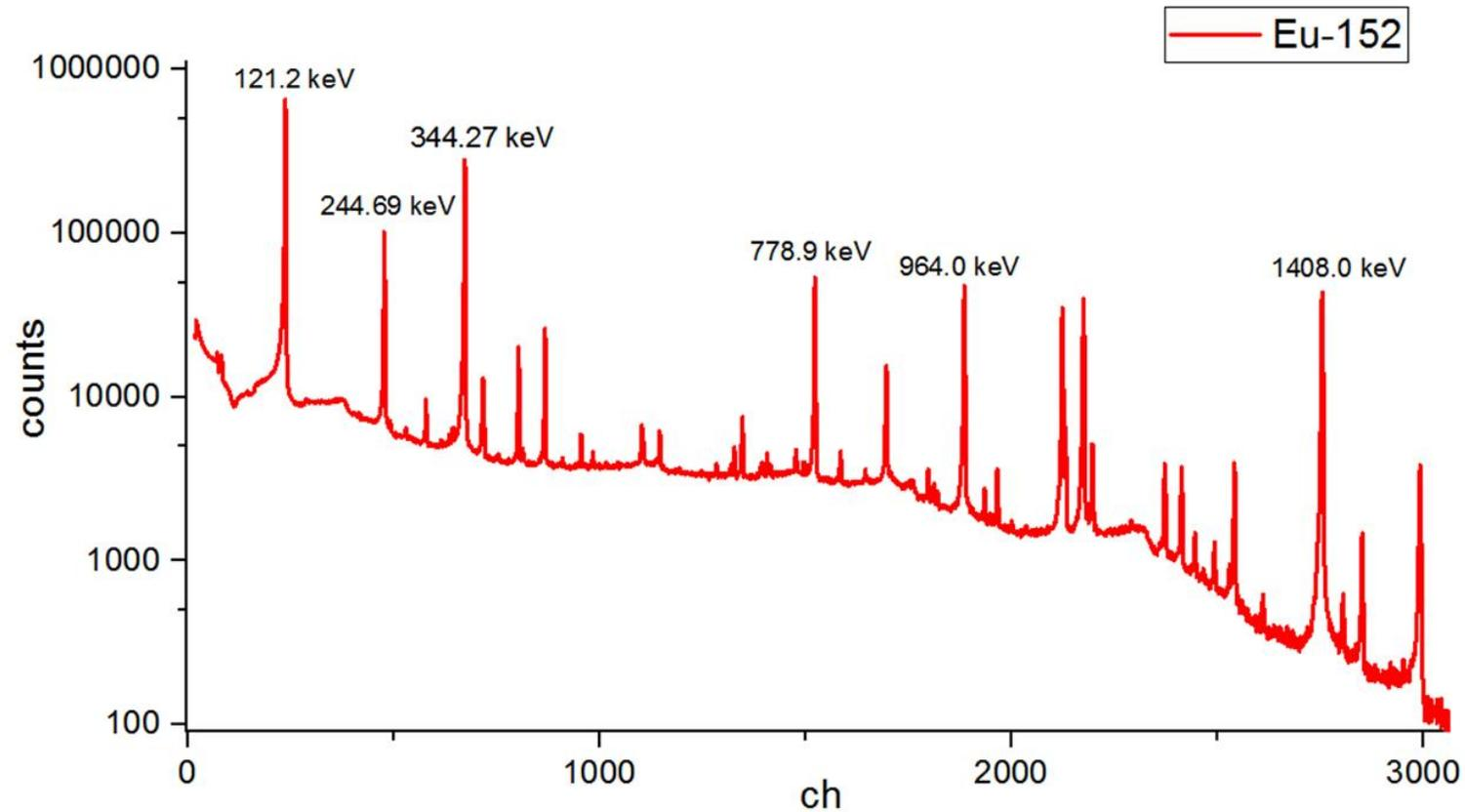
**Figure 5:** 152-Eu energy spectrum registered by a Ge(Li) detector showing energy in keV
