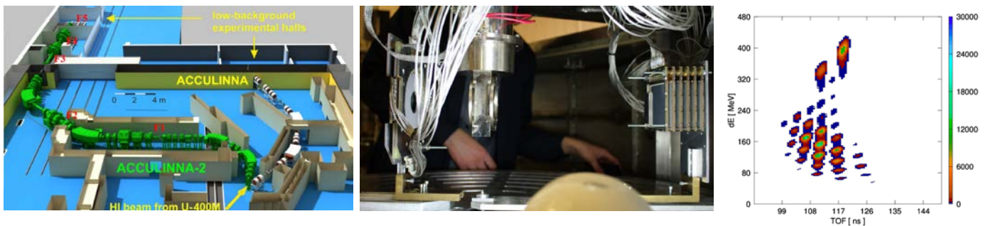
(Left) Main view of ACCULINNA and aACCULINNA-2 separators (center) opened reaction chamber view (right) example of energy lose – Time of Flight spectra
