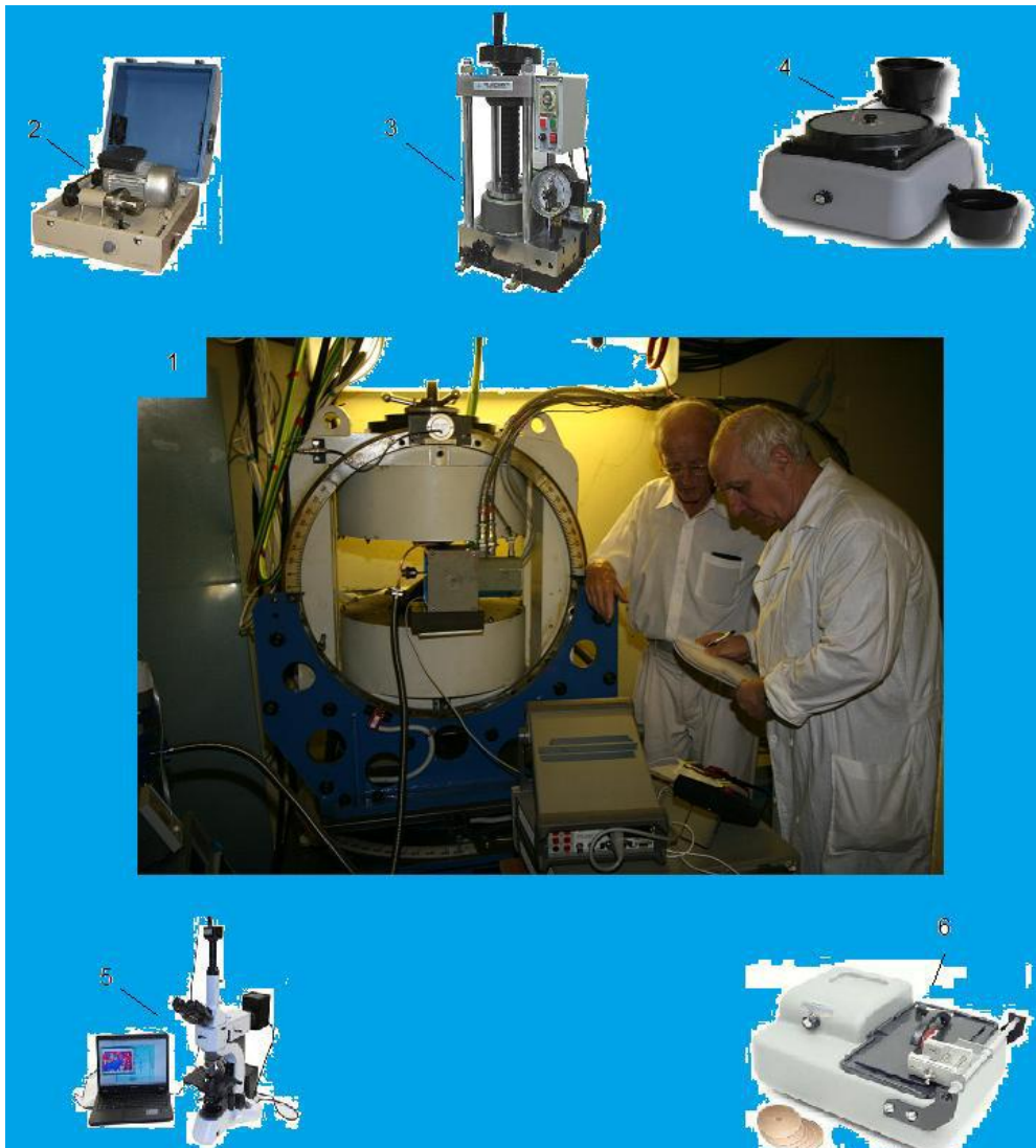
Figure 2 Some instruments used to obtaining manganites and determining their transport properties. 1. General view of installation for magnetoresistance measurements (photo 2008, on YUMO electromagnet; today (2018) installation is in FLNP building); 2. High Speed Vibrating Ball Mill; 3. Electric Hydraulic Laboratory Press; 4. EQ-Unipol-300 Economic 3" Grinder / Polishing; 5. Metallurgical microscope; 6) High Speed Diamond Cut-off Saw
