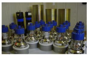
Fig.2. Stilbene modules attached with 3" PMT.
