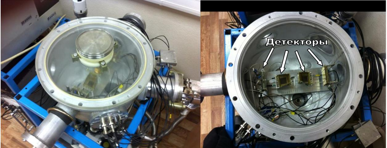
Fig. 3.2. Photo of the reaction chamber and detectors.
