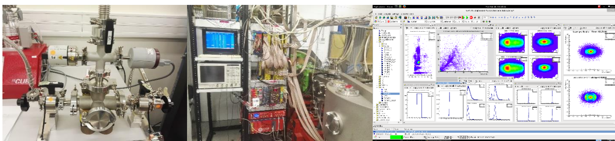
Photographs: flow cell model (on the left); fragment of the data acquisition system for the experiment on the ACCULINNA-2 separator (center); view of the Go4 program window while the acquisition is in progress (on the right).
