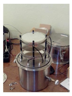
Fig 2. Photograph of twin back-to-back ionization chamber with 235U target mounted on the common cathode.
